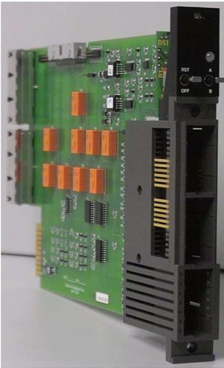
The Mark II Dynaswitch RJ-45 A/B patch/switch module from NSGDatacom is the newest development to the Dynetcom product line. It is designed to enable automatic remote control switching between two primary RJ-45 ports (Active Loop) and two alternate RJ-45 ports (Back-up Loop) for the purposes of communication link restoration, system back up, and alternate routing.
