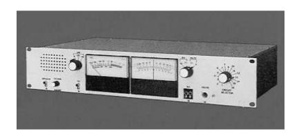
These models provide a db meter for measuring levels, and a speaker for "listening" to the VF analogue data signals. The range is +3 to -30 db in 10 db steps. Input impedance: 10K ohms. An amp-meter is provided for measuring current in neutral or polar current loops (range:  $\pm$  25mA and  $\pm$  75mA; center zero). A selector switch and volt meter enable each lead of the CCITT V.24 digital interface to be measured (range:  $\pm$  5V and  $\pm$  25V; center zero).
