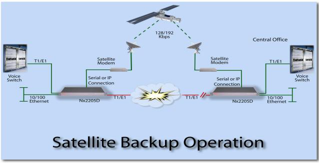
Other benefits provided by the Nx2205D include fractional backup (using proportionally less bandwidth), anti-bounce for channel/circuits prone to brownouts, activity logging and alarming.
